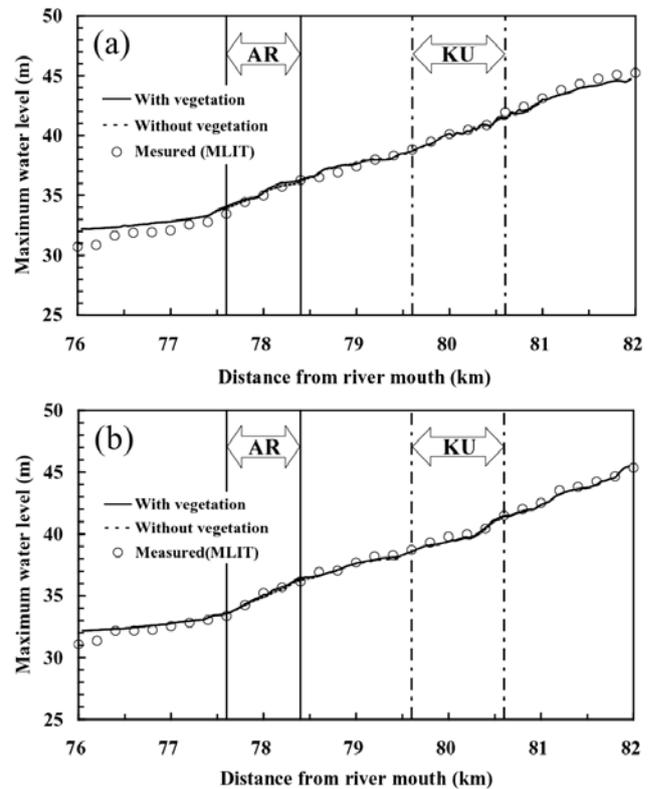
Figure 4 Comparison of simulated and observed maximum water levels along the Arakawa River during the September 2007 flood: (a) on the right bank, (b) on the left bank
