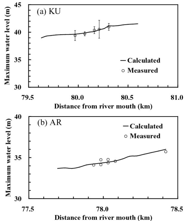
Figure 5 Comparison of simulated and observed maximum water levels along each island during the September 2007 flood: (a) KU, (b) AR. The vertical bars at each point represent the standard deviation.
