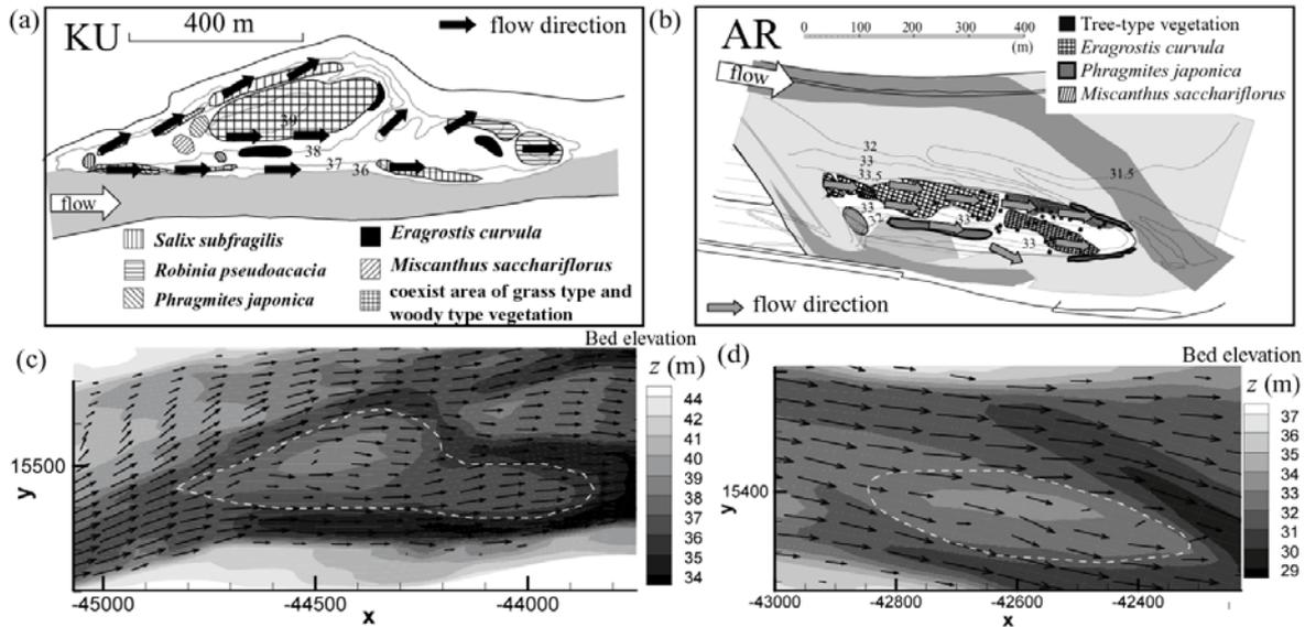
Figure 6 Comparison of simulated and observed velocity vectors of each island during the September 2007 flood: (a) observed velocity vectors at KU, (b) observed velocity vectors at AR, (c) calculated velocity vectors at KU, (d) calculated velocity vectors at AR. The broken lines in (c) and (d) represent the outer shape of each island.
