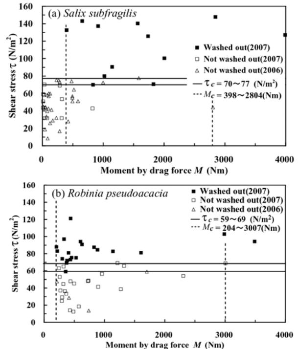
Figure 7 Relationship between moment acting on tree trunks and shear stress at the bed during the September 2007 and October 2006 floods: (a) *S. subfragilis*, (b) *R. pseudoacacia*.  $M_c$ : critical moment for washing out a tree,  $\tau_c$ : critical shear stress at the bed for washing out a tree, closed symbol: trees were washed out, open symbols: trees were not washed out.
