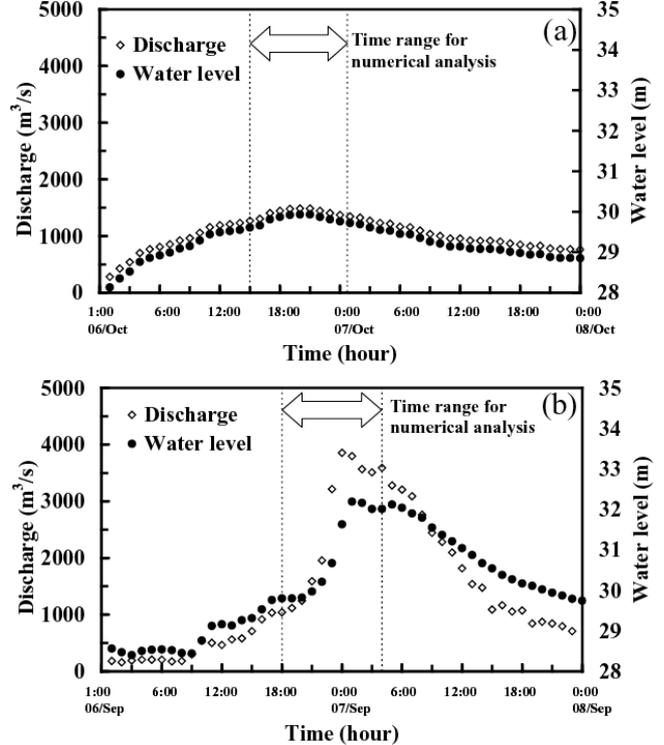
Figure 2 Observed discharge at the Uematsu-bashi gauge station (86 km from river mouth) and water level at the Kumagaya gauge station (76 km from river mouth) used for numerical simulation: (a) October 2006 flood, (b) September 2007 flood
