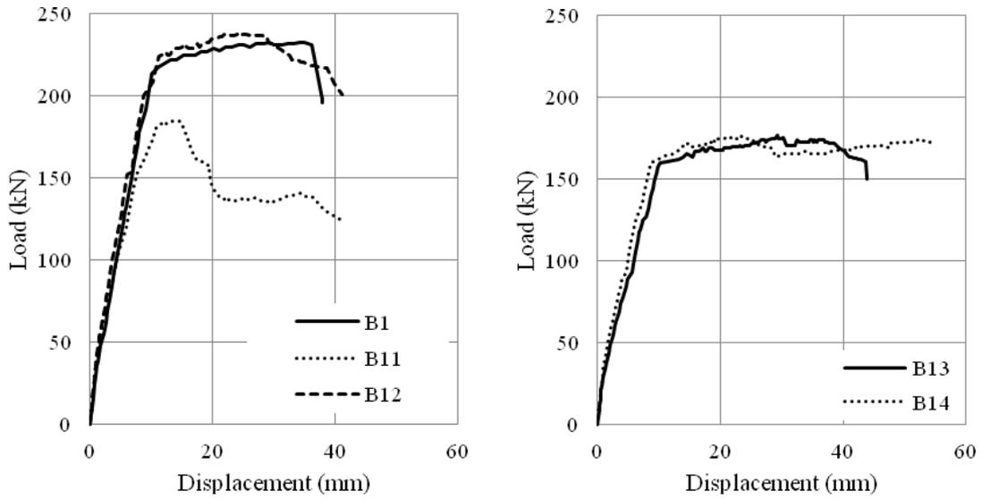
Figure 12. Load-displacement curves of the test beams
