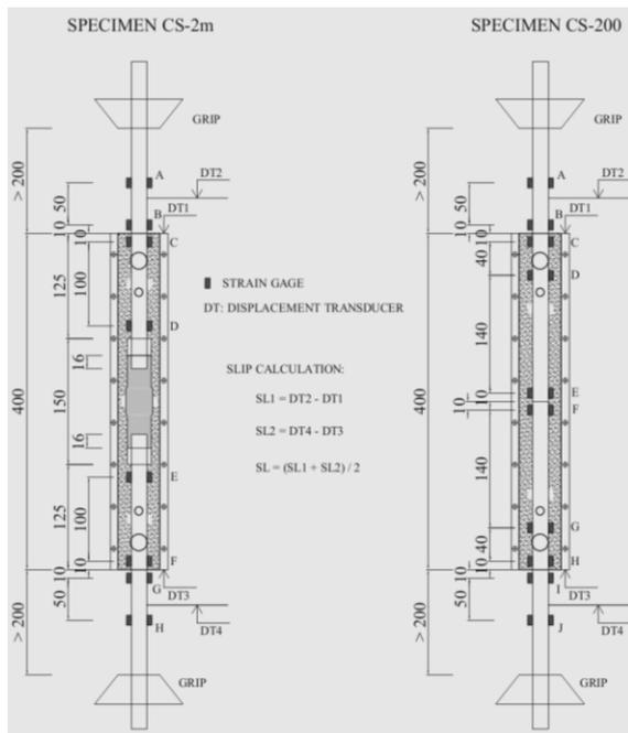
Figure 9. Tensile test setup for the corrective splice
