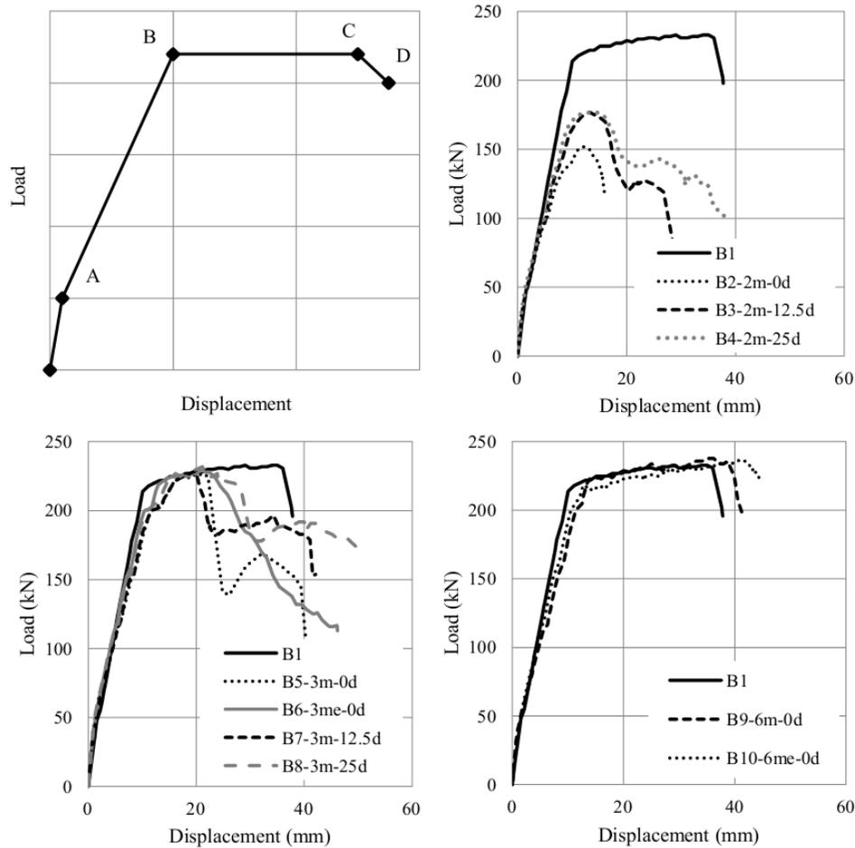
Figure 5. Load-displacement curves of beams
