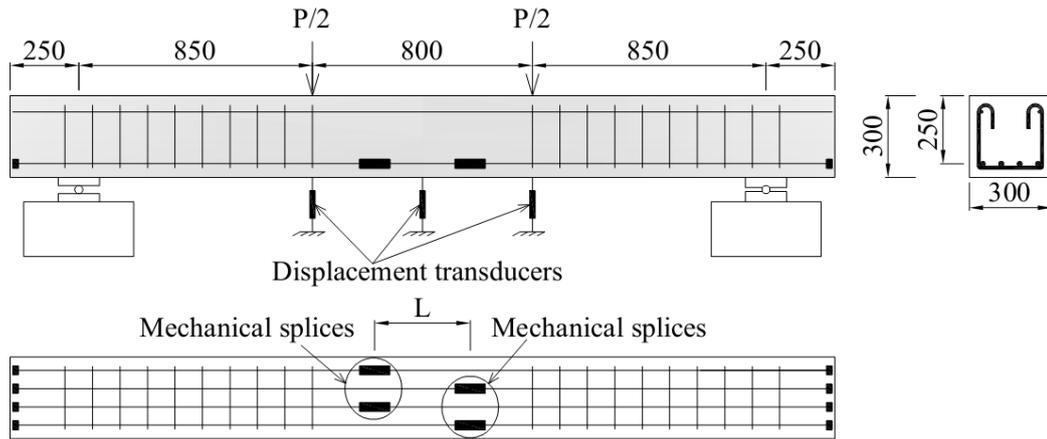
Figure 4. Beam configurations and test set up
