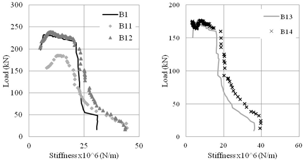
Figure 13. Stiffness of beams using corrective splices
