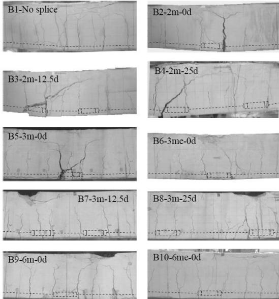
Figure 7. Crack patterns of beams
