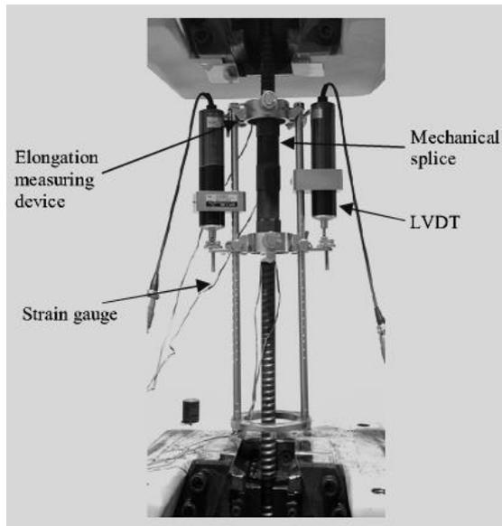
Figure 3. Tensile test set-up
