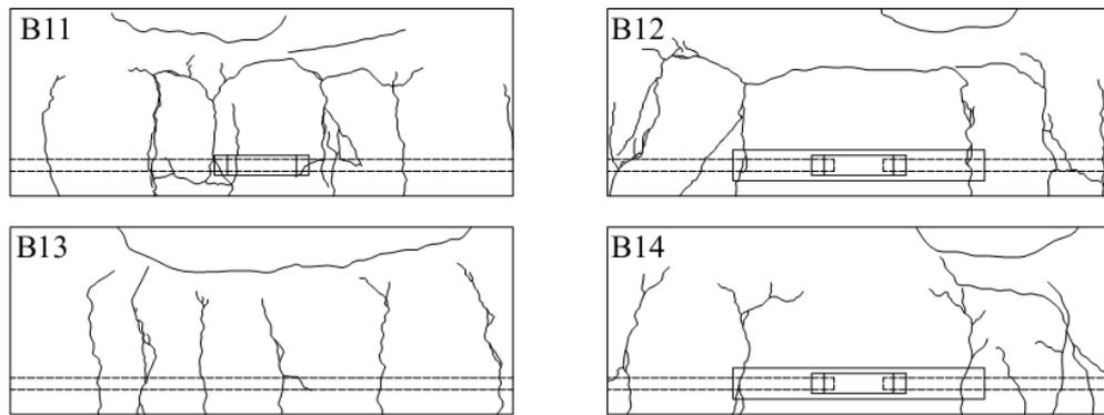
Figure 14. Crack patterns in the corrective splice beam tests
