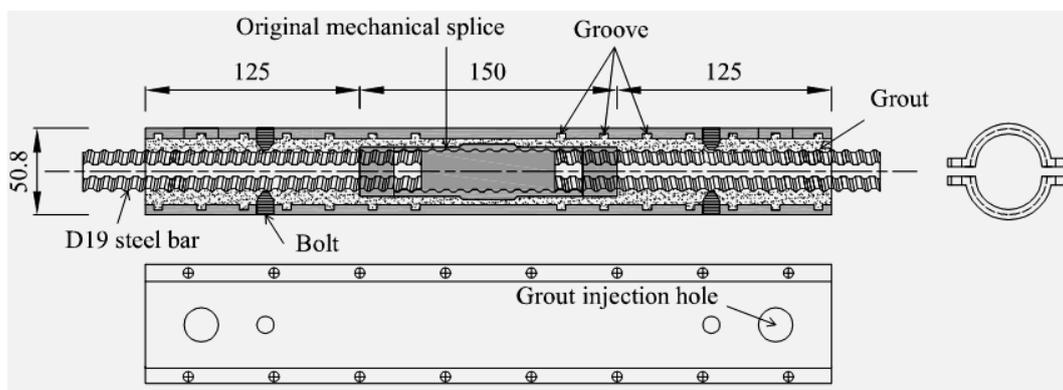
Figure 8. Structure and dimensions of the corrective splice
