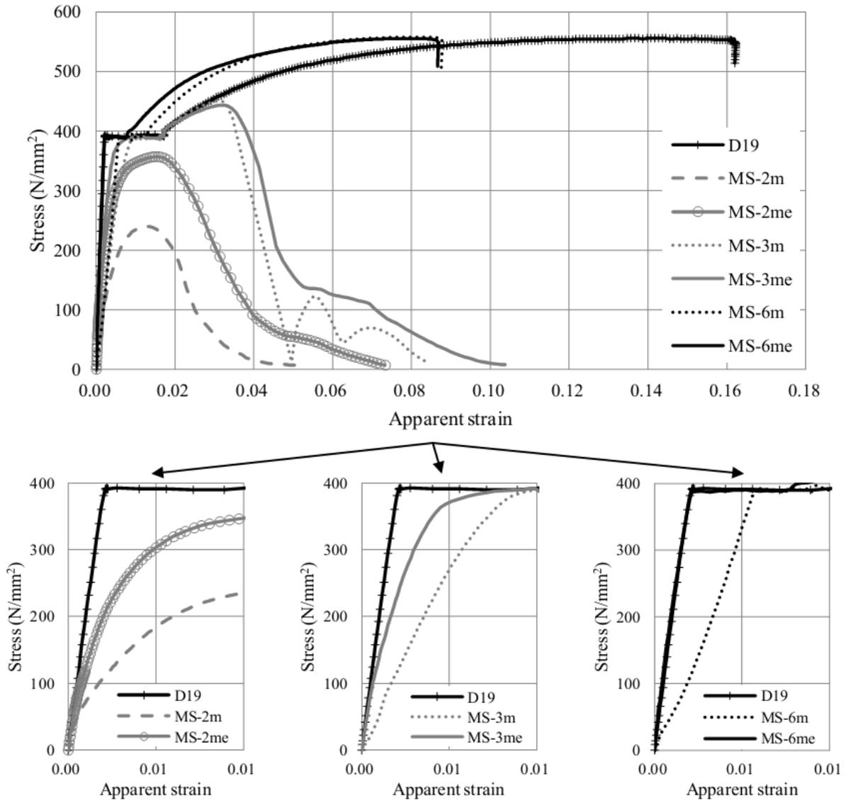
Figure 4. Stress-strain curves of mechanical splices
