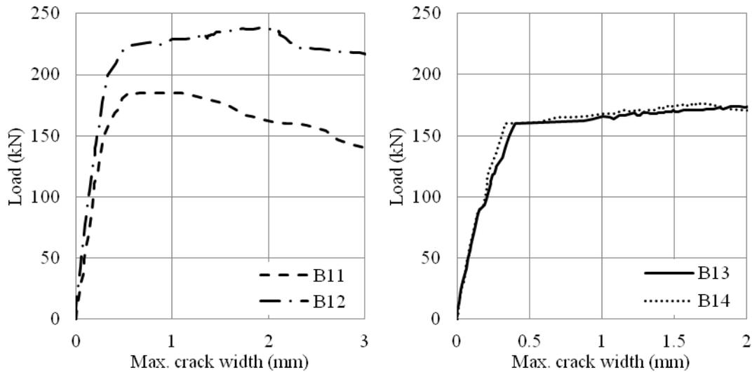
Figure 15. Crack widths development in the test beams
