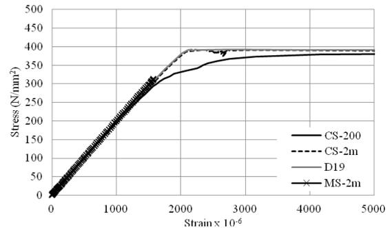
Figure 10. Stress-strain curve of a corrective splice
