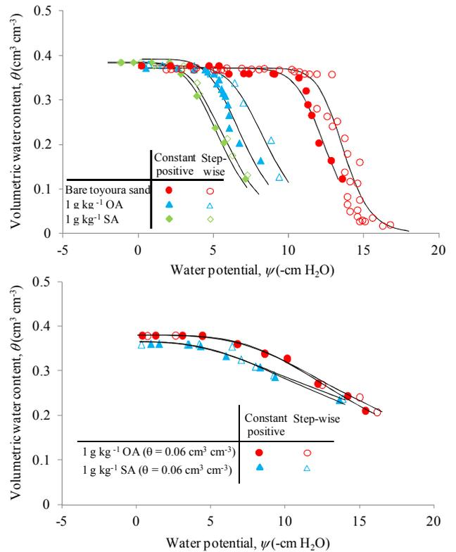
Figure 14 Main wetting curves during step-wise and constant positive pressure imbibition for a) bare (air-dried), OA- and SA- coated Toyoura sand samples ( $1 \text{ g kg}^{-1}$ ), and b) OA- and SA-coated Toyoura sand samples ( $1 \text{ g kg}^{-1}$ ) with 4% initial-water adjusted ( $\theta = 0.06 \text{ cm}^3 \text{ cm}^{-3}$ ). Symbols show measured wetting data and solid lines show curves fitted by the VG (1980) model.
