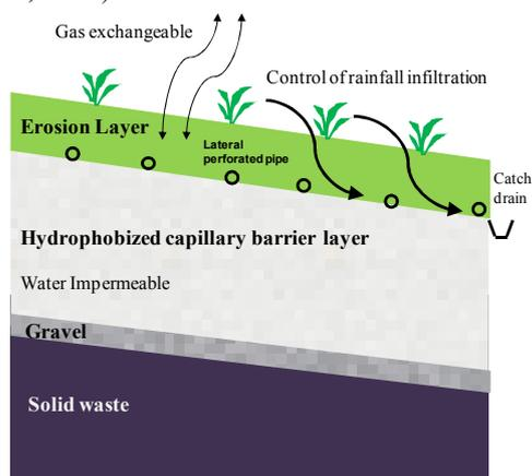
Figure 1 Schematic of hydrophobized capillary barrier layers.
