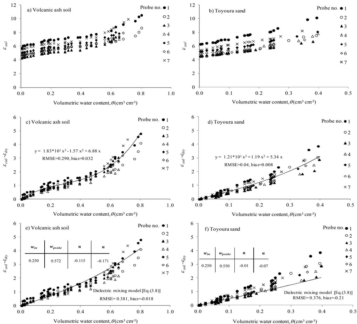
Figure 10 Relationship between dielectric constant,  $\epsilon_{coil}$ , and volumetric water content,  $\theta$ , measured with seven mini T-TDR coil probes for volcanic ash soils (a), and bare Toyoura sand (b). Fitting of Polynomial expression and dielectric mixing model are shown in (c,d) and (e,f) in a normalized  $(\epsilon_{coil}-\epsilon_{dry})-\theta$  relationship, respectively.
