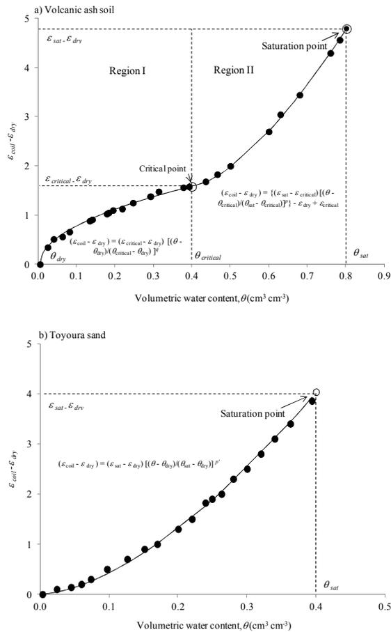
Figure 11 Illustration of proposed calibration model for (a) aggregated volcanic ash soil and (b) single-grained Toyoura sand to describe the relationship between the dielectric constant,  $\epsilon_{coil} - \epsilon_{dry}$ , and volumetric water content,  $\theta$ .
