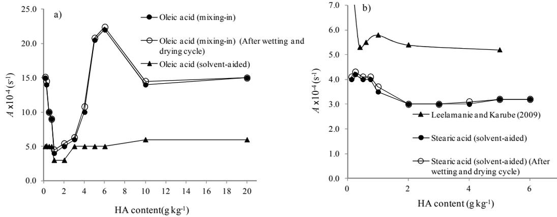
Figure 8 Effect of increasing hydrophobic agent (HA) on coefficient of temporal change in WR,  $A$ , in hydrophobized Toyoura sands before and after the wetting and drying cycle for a) OA (mixing-in) and OA (solvent aided) samples and b) SA (solvent-aided) samples. Note the different y axes.
