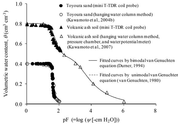
Figure 13 Soil-water retention curves for volcanic ash soil and bare Toyoura sand. The  $\theta_s$  values are plotted at  $pF=0$ .
