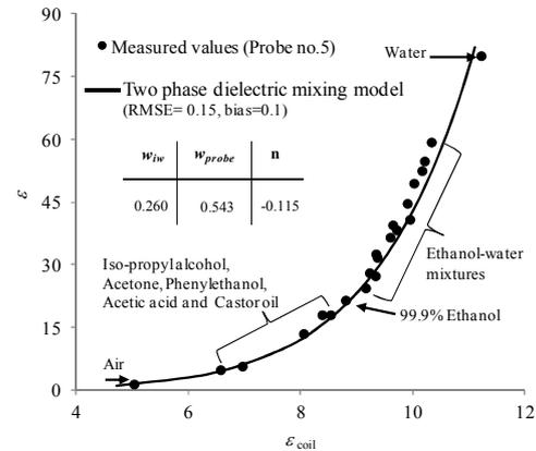
Figure 9 Relationship between apparent dielectric constant measured with a conventional three-rod probe ( $\varepsilon$ ) and a mini T-TDR coil probe ( $\varepsilon_{coil}$ ) in air, water, ethanol, ethanol-water mixtures, iso-propyl alcohol, acetone, phenyl ethanol, acetic acid and castor oil. The solid line shows the two-phase dielectric mixing model fitted to the data points.
