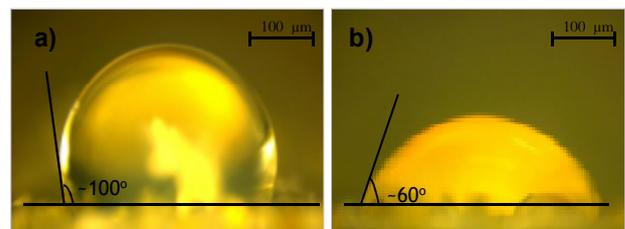
Figure 3 Microphotographs of OA (mixing-in) samples with a)  $100^\circ$  contact angles for  $t=0\text{s}$  and b)  $60^\circ$  contact angle for  $t=900\text{s}$  obtained from the SDM
