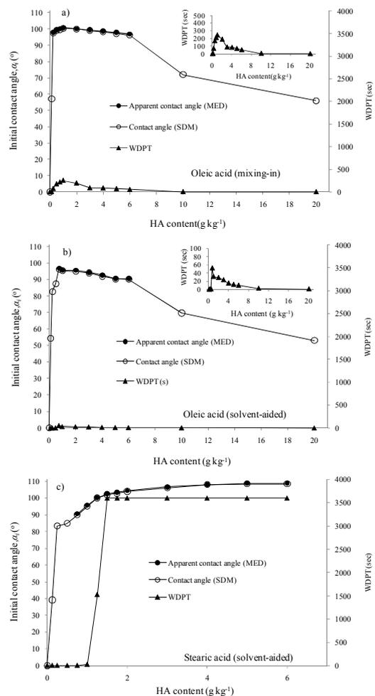
Figure 6 Initial contact angles,  $\alpha_i$ , measured as a function of HA content by the MED test and the SDM for a) oleic acid (mixing-in), b) oleic acid (solvent-aided) and c) stearic acid (solvent-aided) samples. Results from the WDPT test are also shown. Note that the x-axis used in (c) is different from those in (a) and (b).
