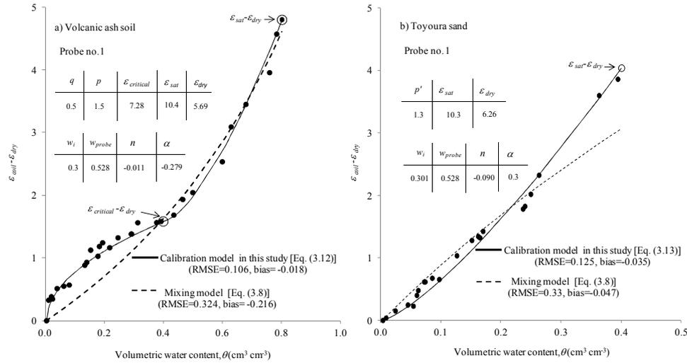
Figure 12 Calibration model fitted to the normalized dielectric constant,  $\epsilon_{coil}-\epsilon_{dry}$ , and volumetric water content,  $\theta$ , relationship measured with mini T-TDR probe no. 1 for (a) volcanic ash soil and (b) Toyoura sand.
