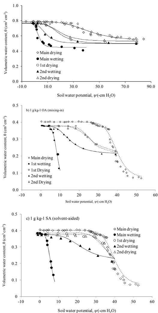
Figure 15 Volumetric water content,  $\theta$ , as a function of water potential,  $\psi$ , for (a) VAS (air-dried), (b) OA-coated, and (c) SA-coated Toyoura sand samples (1 g kg<sup>-1</sup>).
