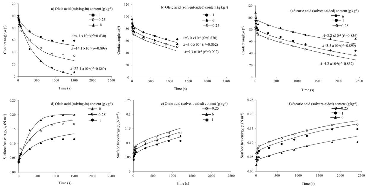
Figure 7 Contact angles,  $\alpha$ , and soil surface free energy,  $\gamma_s$ , as a function of soil-water contact time for a) and d) oleic acid (mixing-in), b) and e) oleic acid (solvent-aided), and c) and f) stearic acid (solvent-aided) samples.
