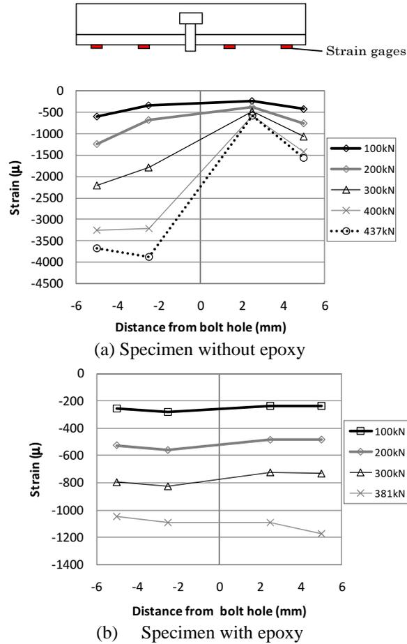
Figure 17 Strain distribution in HFRP top flange near bolt hole
