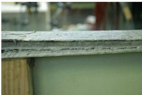
Figure 5 Closer view of delamination
