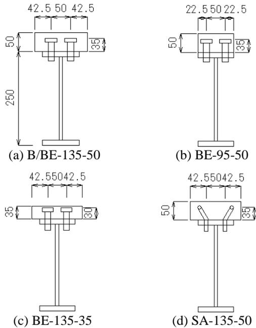
Figure 12 Dimensions of the beam cross-sections
