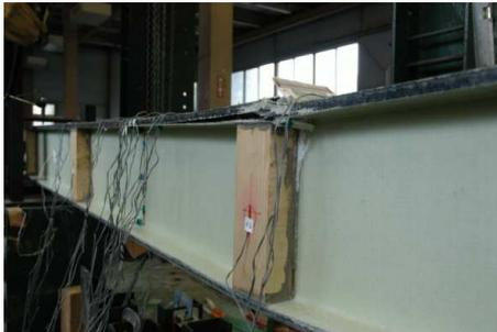
Figure 4 Crushing of fibers and delamination
