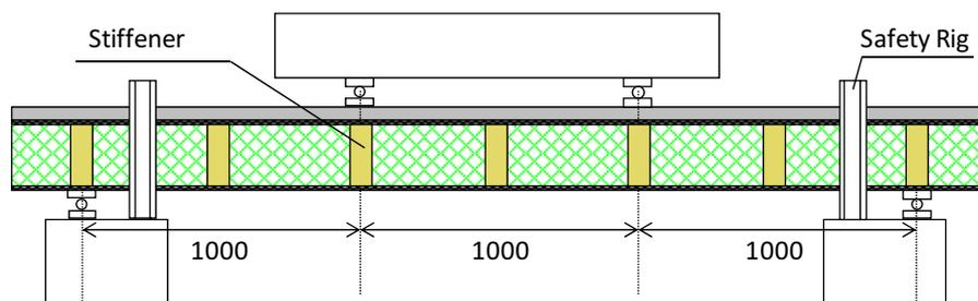
Figure 11 Geometry of specimen for flexural test
