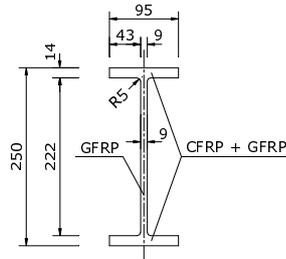
Figure 1 Dimensions of HFRP I-beams (mm)
