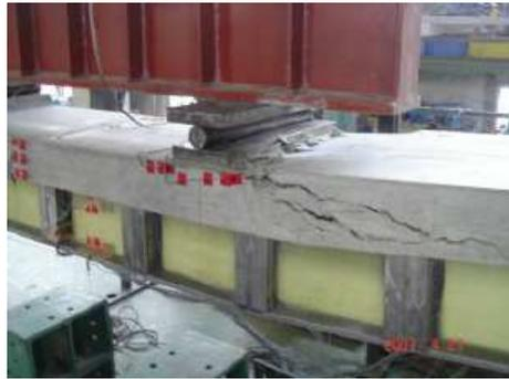
(a) Compression failure of NSC slab
