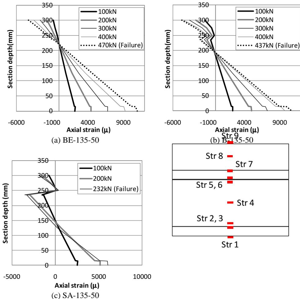
Figure 16 Longitudinal strain distribution along the depth of the composite beam
