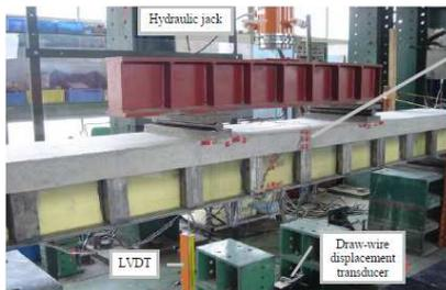
Figure 8 Test setup of HFRP-NSC
