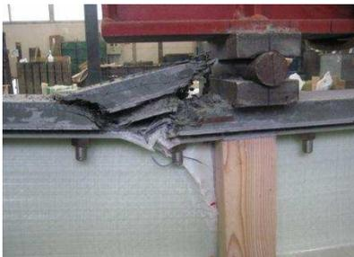
(a) Crushing of UHPFRC slab
