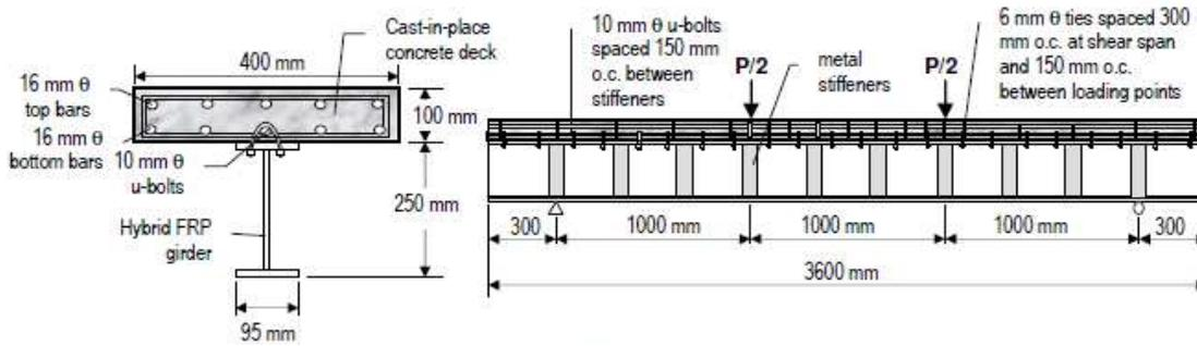
Figure 7 Dimensions and configurations of specimen HFRP-NSC
