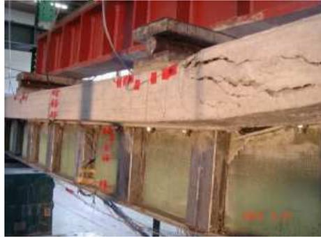
(b) Shear failure of HFRP beam
