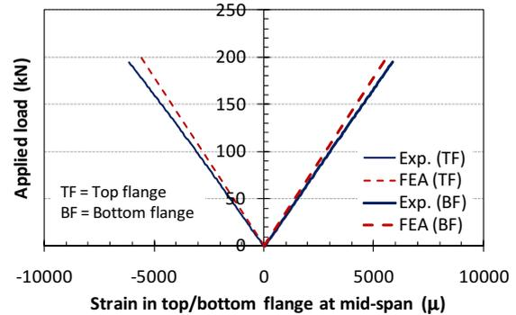
Figure 6 Load-longitudinal strain curve
