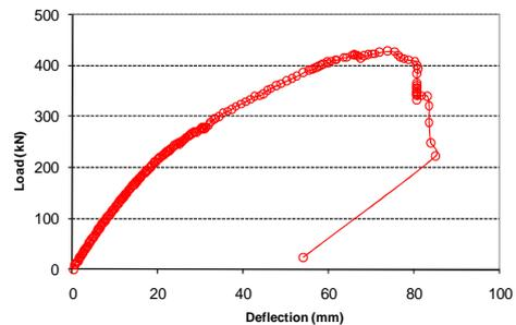
Figure 9 Load and middle span deflection curve of HFRP-NSC
