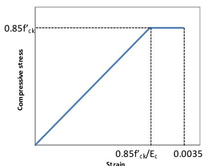
Figure 19 Bi-linear stress-strain relationship of UHPFRC
