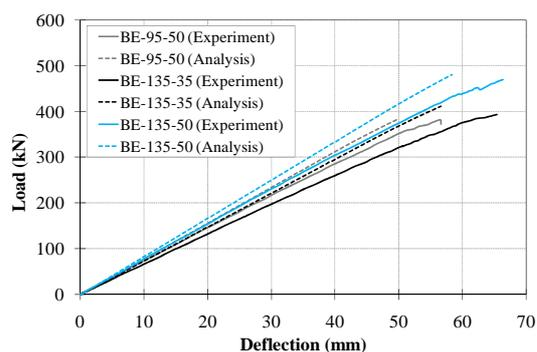
Figure 20 Comparisons of load-deflection curves between experiments and analysis
