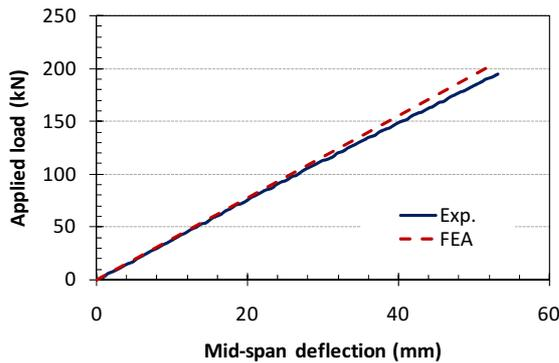
Figure 3 Load-deflection curves at mid-span section
