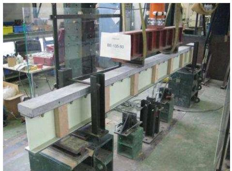
Figure 14 Flexural beam test setup
