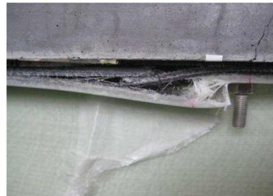
(b) HFRP flange delamination failure
