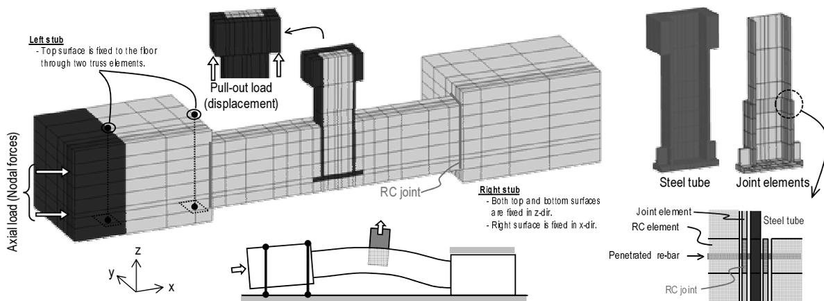
Fig.7 Finite element model used in the simulation of pull-out test
