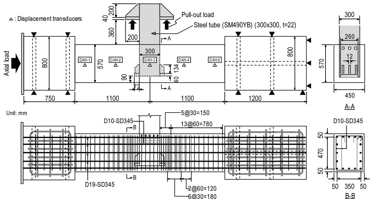
Fig.4 Dimensions and reinforcement arrangement of test specimen
