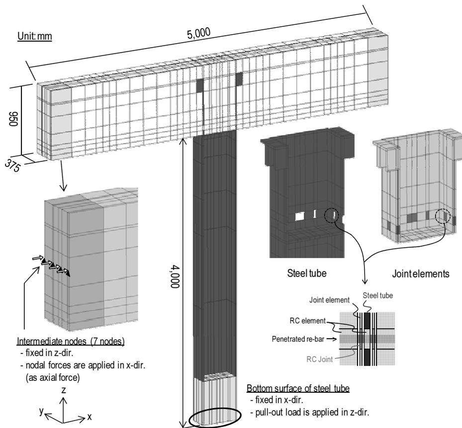
Fig.9 Finite element model used in the simulation of joint connection in the actual bridge
