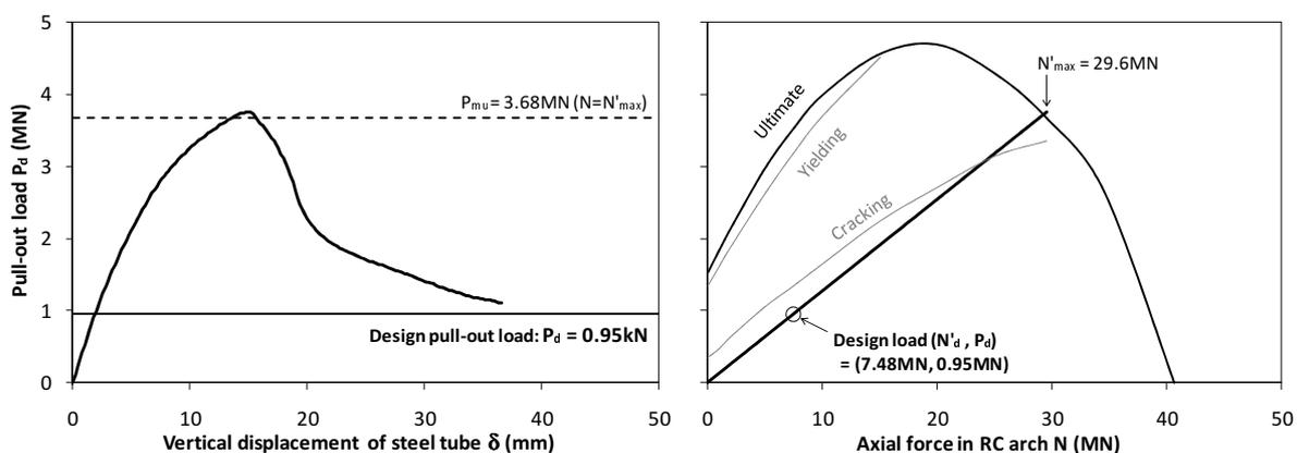
**Fig.11 Pull-out load and displacement relationship and the interaction curve of arch section**
