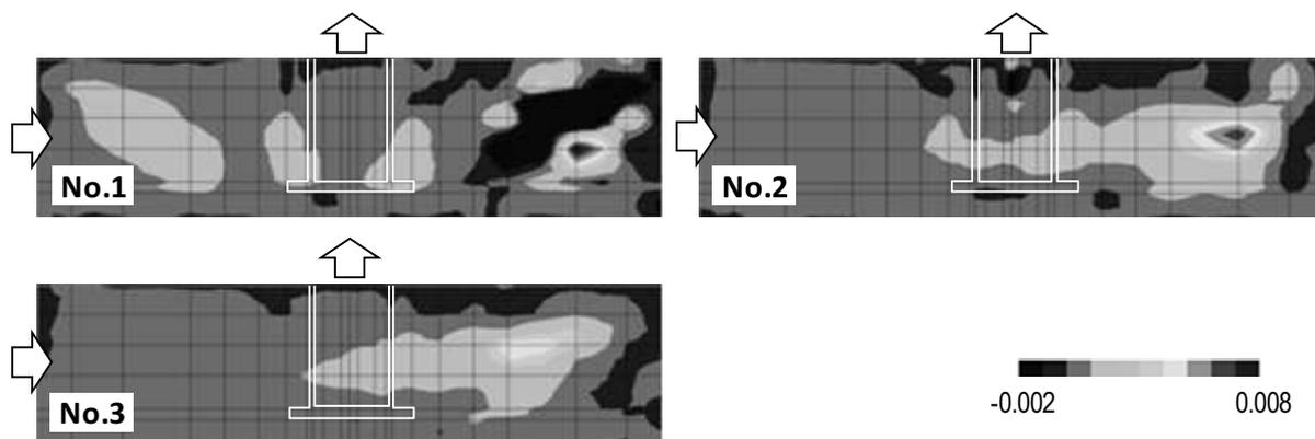
Fig.8 Vertical strain contour plots of the specimens
