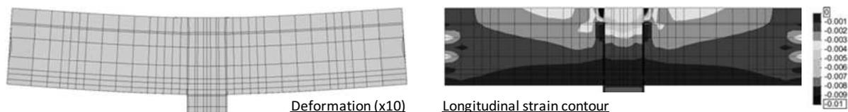
**Fig.10 Deformation and longitudinal strain contour plot when the maximum load was reached**
