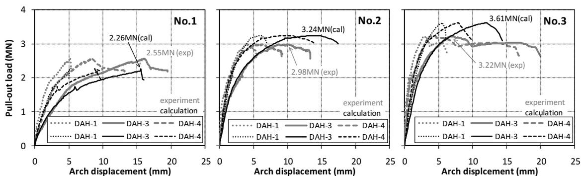
Fig.6 Relationships between pull-out load and arch displacement
