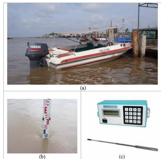
Fig. 4 Wave measurement equipment (a) Boat used for wave generation, (b) Staff gauge and, (c) Electromagnetic velocity device.
