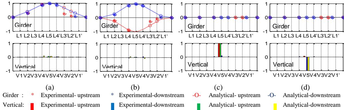
Fig.7. Experimentally identified vibration mode shapes from FV1: (a) first symmetric vertical; (b) first symmetric torsional; (c) V5u vertical member local; (d) V5d vertical member local.
