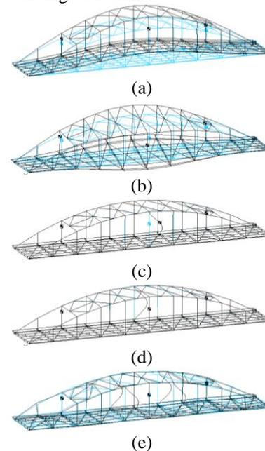
Fig.2. Numerically analyzed vibration modes of the arch bridge with moveable support conditions: (a) first symmetric vertical; (b) first symmetric torsional; (c) V5u vertical member local; (d) V5d vertical member local; (e) V4 vertical member coupled.
