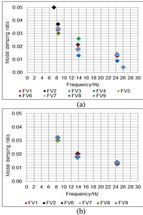
Fig.11. Variation of natural frequency vs modal damping ratio of Bridge III: (a) after second step of screening; (b) after third step of screening.
