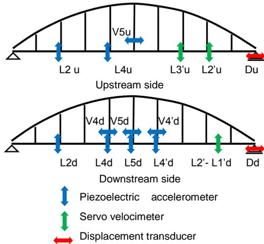
Fig.3. Position of accelerometers, velocimeters and displacement transducers placed during field vibration measurements of the arch bridge.
