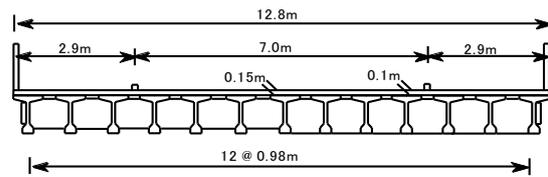
Fig.8. Typical section of PC Bridges (Bridge III).
