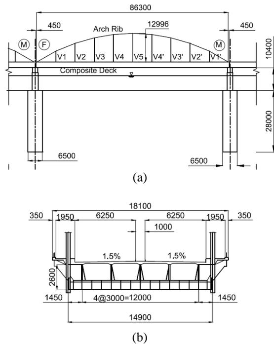
Fig. 1. Studied Langer-type arch bridge constructed in 1971: (a) elevation of bridge; (b) section of the deck. (Unit in millimeters)
