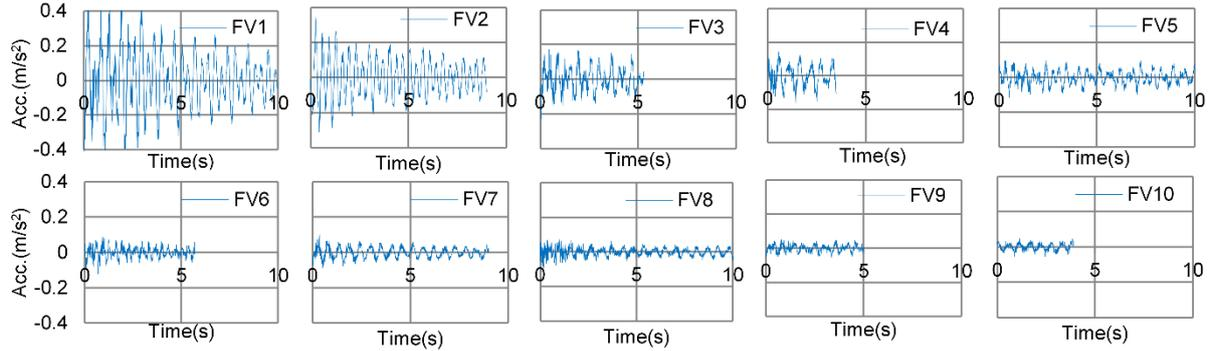
Fig.4. Free vibration time histories of bridge deck measured at L5d for all sets of FV records.
