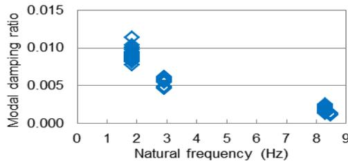
Fig.5. Relation of screened natural frequencies and modal damping ratios from FV1.
