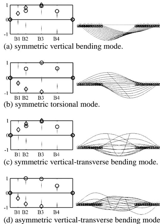
Fig.10. Comparison of experimental and analytical mode shapes of Bridge III.
