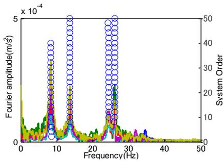
Fig.9. Spectrum and system identification-Bridge III (FV 9).
