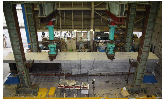
Fig.13-Loading Test of 1/2 Scaled Model
